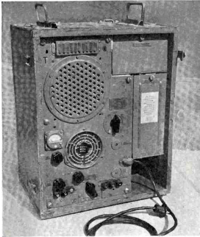
Knob near center controls a variac for choice of 110-220 v.
