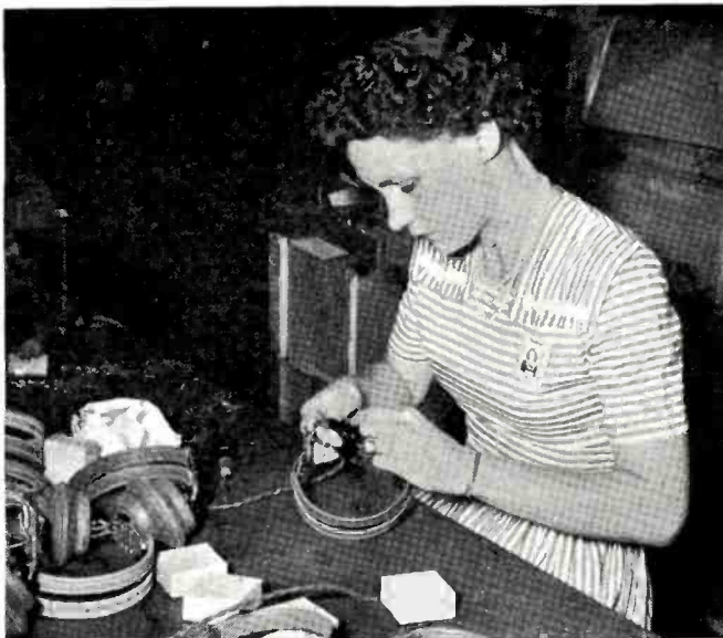
Worker at the Philadelphia Signal Depot repairing radio head-set.
