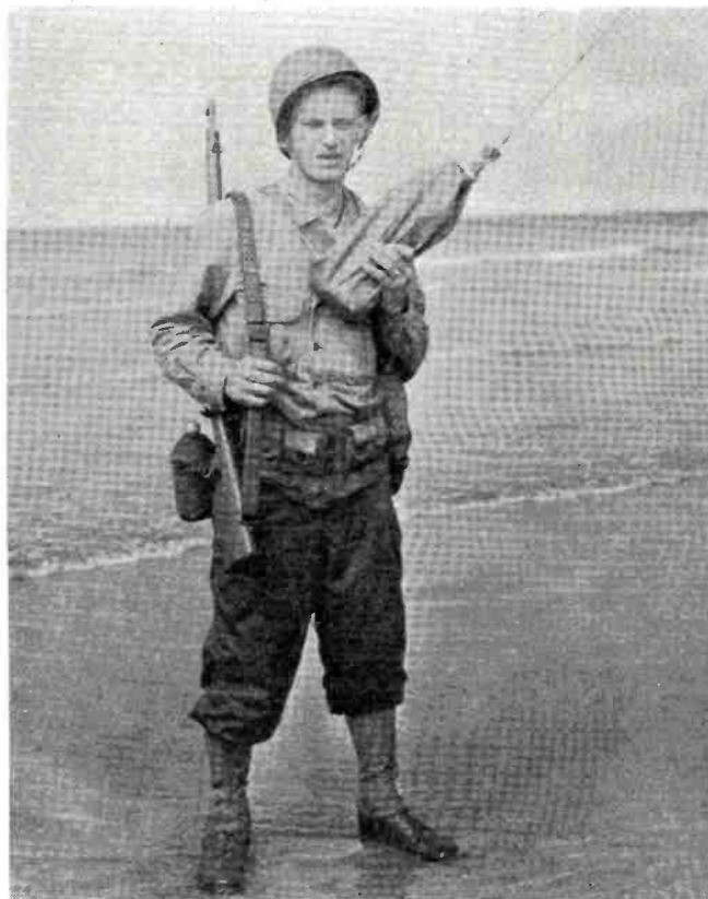
Waterproofed handie-talkie after receiving wade test. Each antenna connection is waterproofed with a special compound.
