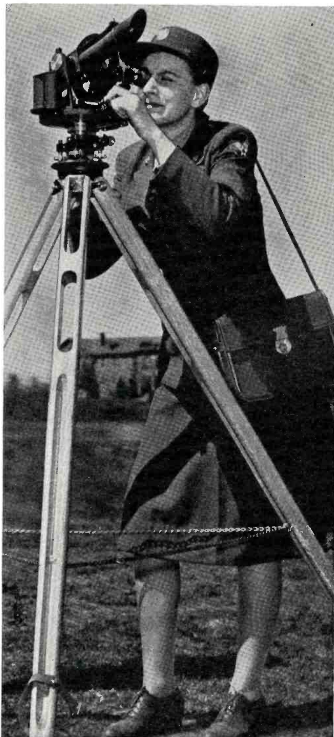
Theodolite being used to record the wind velocity and direction.
