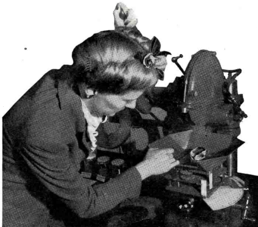
Signal Corps technician using diamond saw to cut raw quartz crystals. Water-like sheets are produced and used as oscillators in many types of radio equipment.
