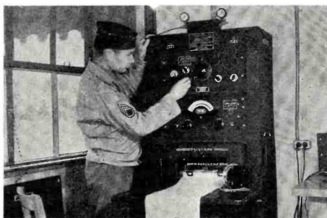
Trained operator tuning in on radiosonde equipment for latest data on pressure, temperature, and humidity of the upper air.
