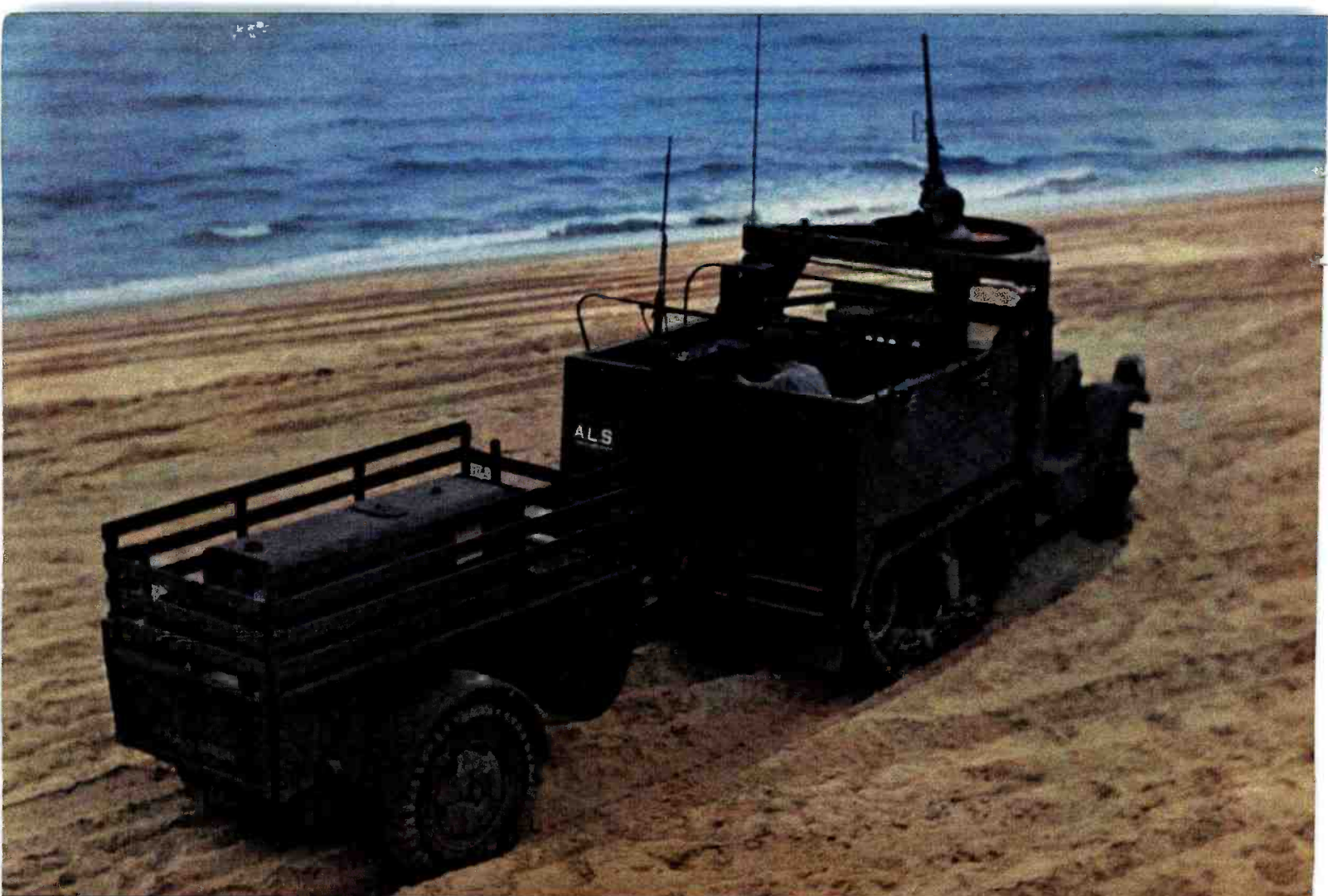
↑ SCR-299 mobile transmitter installed in half-trac. This unit travels easily over sand and rough ground.
