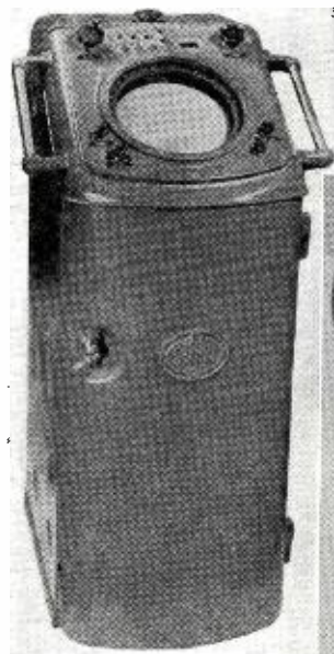
Indicator binnacle of the Sperry Gyroscope set houses 12" PPI and associated controls. Visible are range selector switch, variable range marker, bearing cursor, anti-clutter selector switch, and azimuth scale illumination control.
