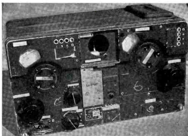
Left to right: Receiver, Modulator and Transmitter units.
