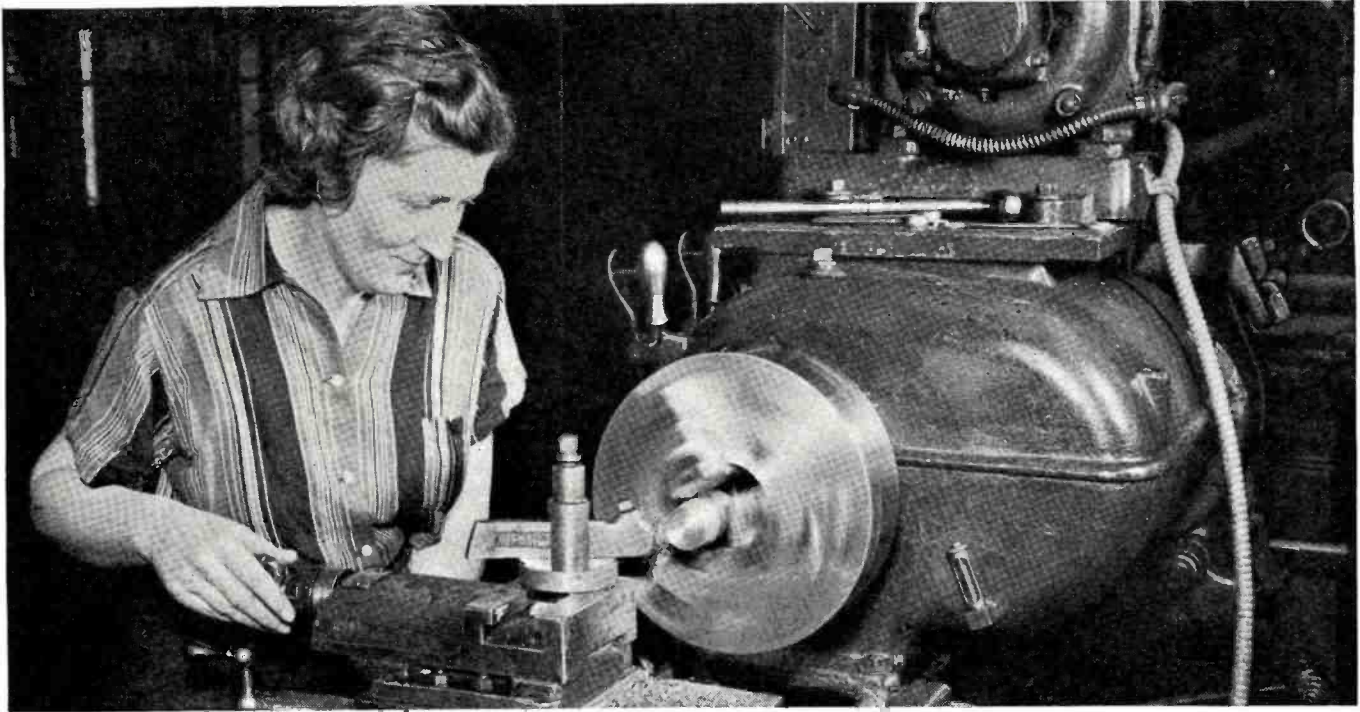
Signal Corps laboratory assistant performing a shaft-turning operation on a lathe at Fort Monmouth.
