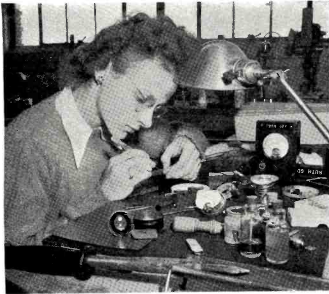
Repair Shop—operator making adjustments on electrical meters.
