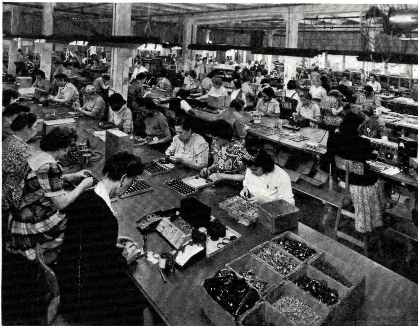
Typical radio-assembly plant laid out for high-speed production. T17 microphones are being assembled, inspected, and tested.
